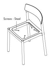
2. Unscrew the bolts located inside the frame of the seat. This can be done with a socket wrench.
