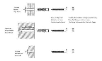
Template for drilling for mounting screws.
